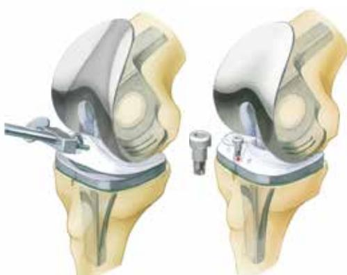
The UHMWPE plateau is pressed down and fixed into place by the self-locking fixation screw.
